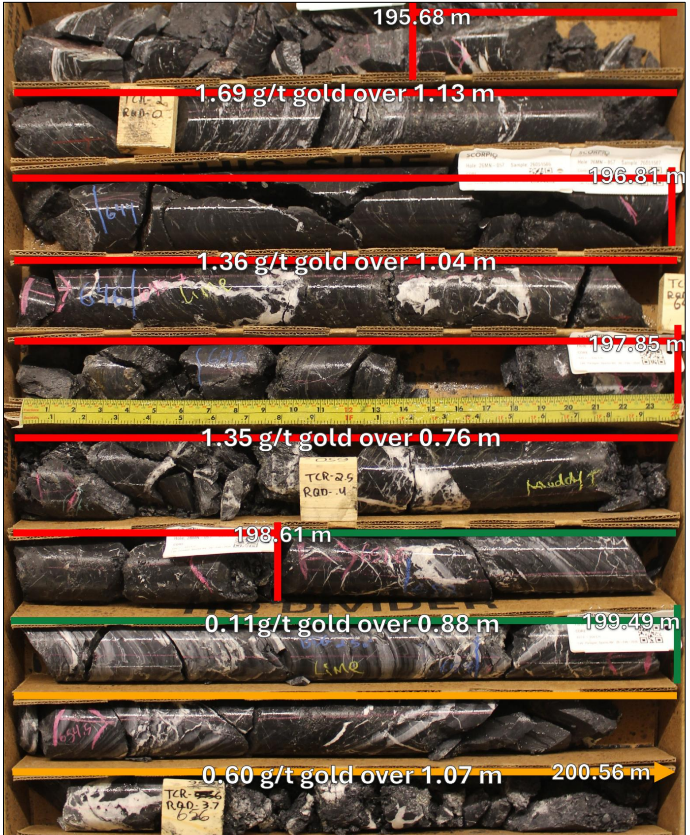
Figure 4. Drill hole 26MN-057, interval 195.68 to 200.56 m, displaying Ordovician Zanzibar Formation limestones with quartz-calcite-adularia epithermal veins.
