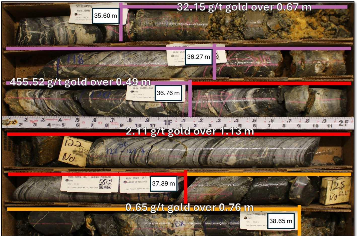
Figure 4. Drill hole 26MN-067, interval 35.60 m to 38.65 m, displaying Ordovician Zanzibar Formation limestones with oxidized quartz-calcite-adularia epithermal veins.
