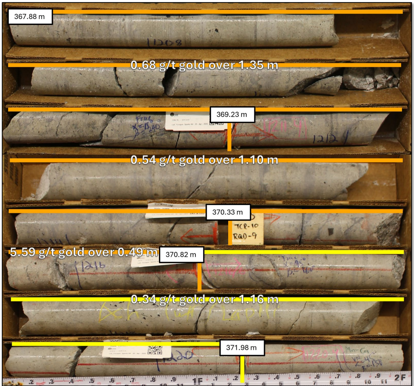
Figure 5. Drill hole 26MN-078, interval 367.88 m to 371.98 m, displaying mineralized volcanic tuff units within the Oligocene Round Rock Formation.
