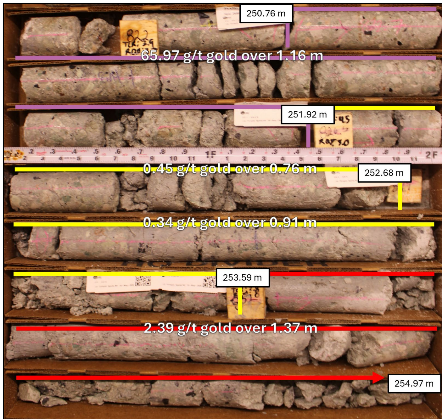
Figure 5. Drill hole 26MN-091, interval 250.76 m to 254.97 m, displaying mineralized volcanic tuff units of the Oligocene Round Rock Formation.
