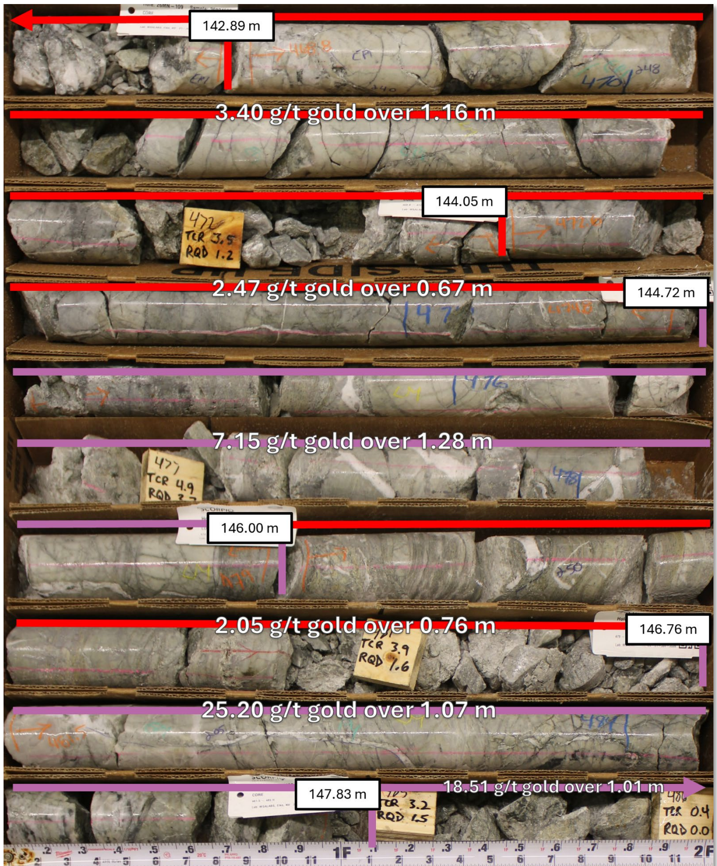
Figure 3. Drill hole 26MN-109, interval 142.89 m to 147.83 m, displaying Cambrian Gold Hill Formation brecciated and silicified marble with quartz-calcite epithermal veins.
